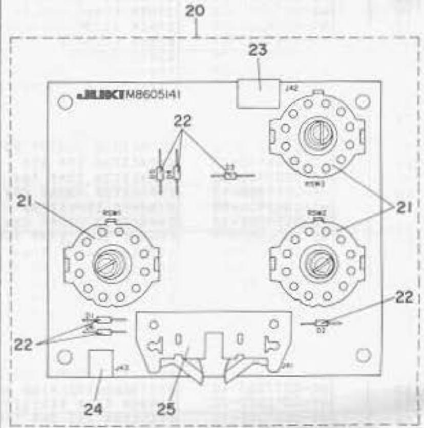
16. INPUT, OUTPUT CIRCUIT BOARD ASSEMBLY
